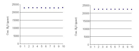
The water concentration measurements made throughout the series shows that every injection is consistent even in the presence of growing salt concentration, see Figure 1.
