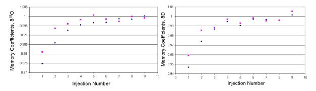
Figure 3. Left hand side data shows the values obtained for  $\delta^{18}O$  memory. Right hand data shows the values obtained for  $\delta D$  memory. For both charts, the blue diamond  $\bullet$  represents the first transition from the tap water to the enriched sample and the pink square  $\blacksquare$  represents the last transition, many hundreds of samples later. The memory is unaffected by the salts load.
