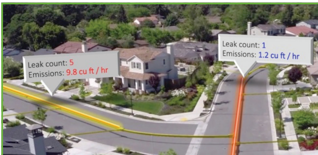
Figure 1. Emissions Quantification and Leak Density Estimation concept. If two pipelines incur similar replacement capital expense, but only one can be replaced in a given year, significant future O&M expense can be avoided by using capital dollars to replace the most leak-dense section. Traditional models can benefit from the addition of methane data to improve their performance in maximizing this capital efficiency.
