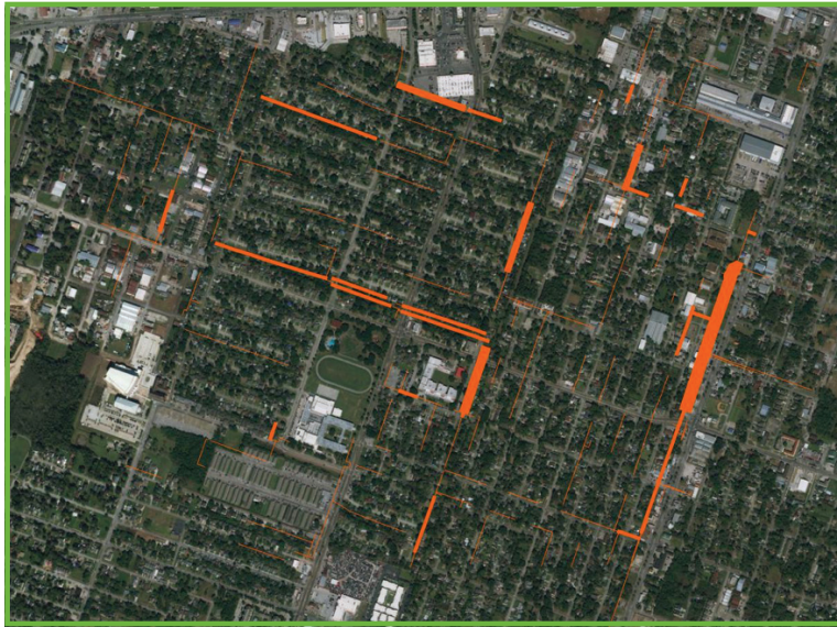
Figure 2. Pipe sections prioritized by Picarro's Emissions Quantification Analytics where thick lines show the highest leak density of pipe segments. Leak density is calculated by analytics that process Picarro's methane emissions measurements along each section.
