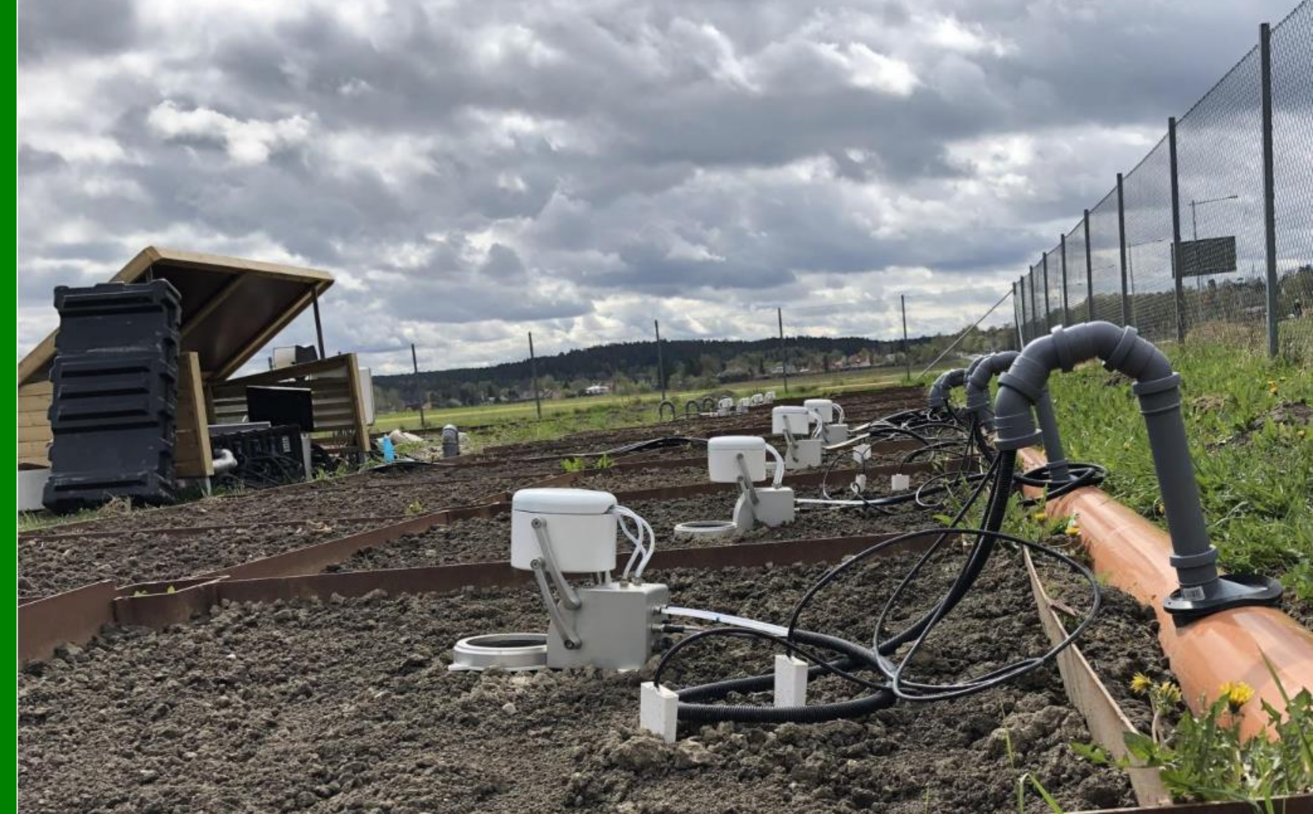
Fig. 1: Schematic illustrating the integration of the G5131- i and G2201- i analyzer with a multiplexer and a eosAC automated chamber system. The G5131- i is subsampling air from the G2201- i recirculation loop (also see box on 'Considerations for soil chamber measurements').
