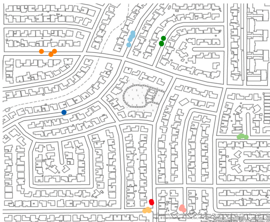
Fig. 3. Example of geospatial clustering to associate one or more detections with a source. Each point represents the location where a single plume was detected. Measurements that are clustered together are shown by like colors. (For interpretation of the references to color in this figure legend, the reader is referred to the Web version of this article.)
