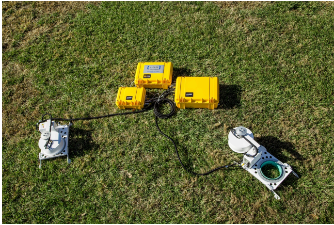
Figure 7. A multiplexed LI-8100A System deployed with the Los Gatos Research Ultra-Portable Greenhouse Gas Analyzer (model 915-0011).
