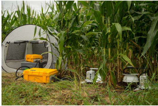
Figure 11. A multiplexed LI-8100A System deployed with the Picarro G2508.
