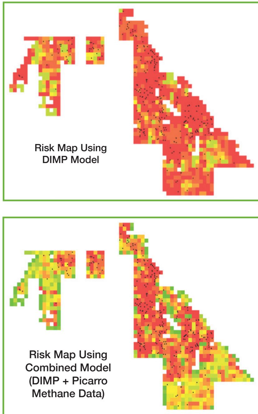
Figure 2. Subset of 4000 miles dataset. Example maps showing the performance of the DIMP and Combined models. Risk per map tile is indicated by color (red=high risk) and leaks found during subsequent compliance survey are indicated by black dots.
